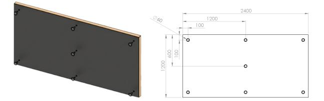
When fixing the panel to the soffit, start with the centre fixing, this will help support the weight of the board while the remaining fixings are installed.
