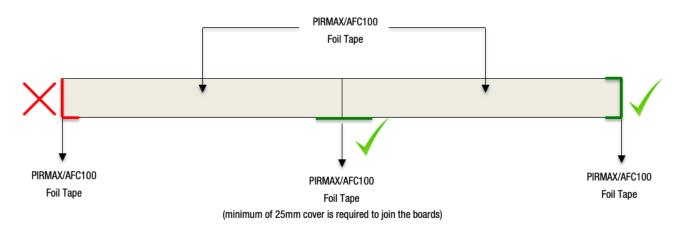
4. Wrapping of the centre joints requires equal tape cover along each edge using the **PIRMAX/AFC100** (100mm) reinforced self-adhesive tape. In all cases, a minimum of 25mm coverage from the edge of the panel is required.
