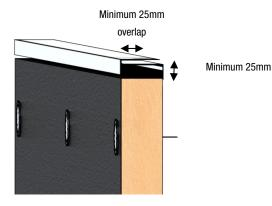
5. Where the **ISO<sup>2</sup> Pane**I is more than 50mm thick, the **PIRMAX/AFC100** will not be wide enough to satisfy the minimum 25mm adhesion width to the foil surfaces of the paneI. In these instances, two lengths of the **PIRMAX/AFC100** will need to be overlapped by a minimum of 25mm to create a wide edge tape.
